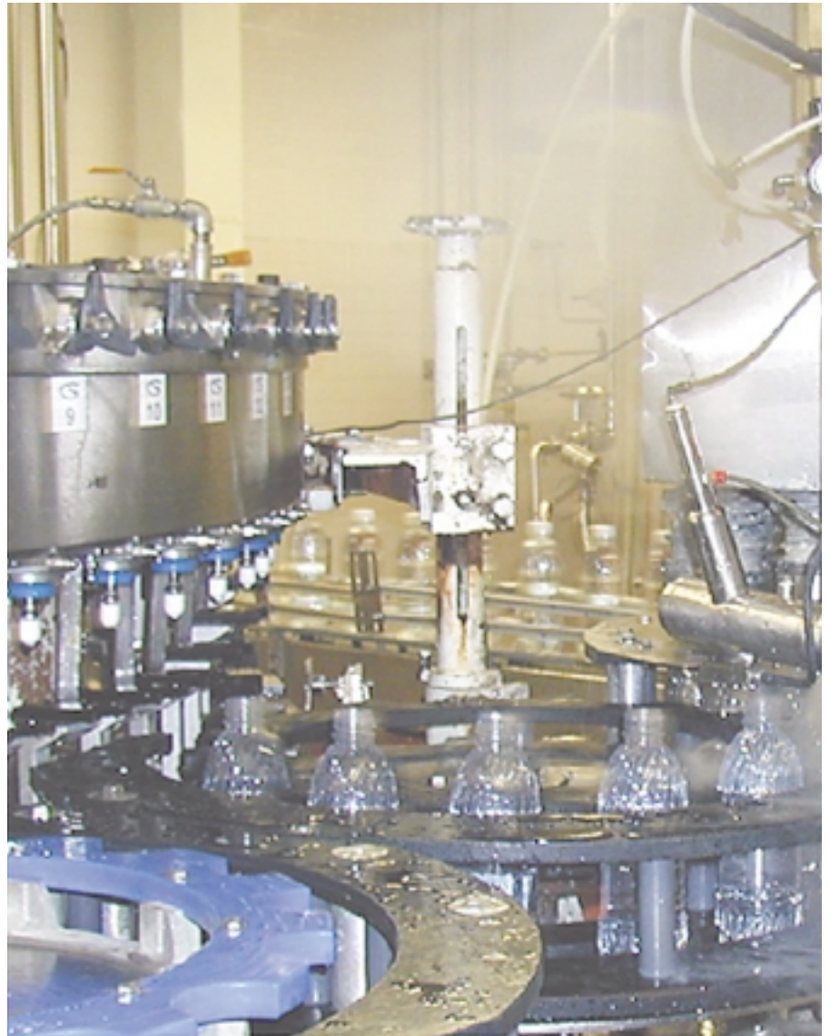
Vacuum-jacketed liquid nitrogen injection provides consistent pressurization when packaging water in lightweight bottles.
