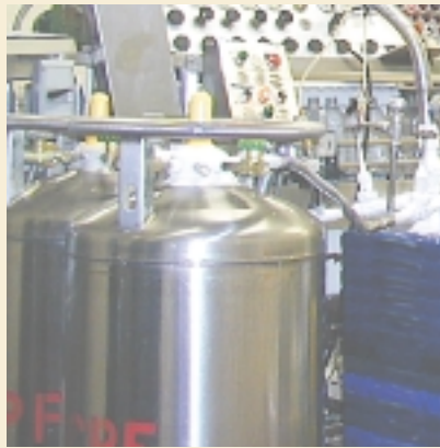
Both portable dewars and bulk tank-fed systems can be used with nitrogen dosing systems. Because of their size, portable dewars (left) must be refilled regularly, but bulk tank systems (right) do not.
