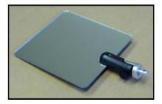
**Flash Light**: To be able to illuminate the surface being swabbed. Light weight, LED.
