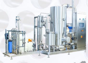
STMC models produce sterile WFI virtually with any type of water supply, thanks to many water pretreatment technologies, integrated on the same skid of the machine.
