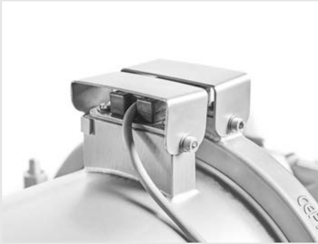
Coded sensors at the removable parts Ensures that equipment is fully assembled and secure in use, sensors are in matched pairs and circuit must be complete prior to operation
