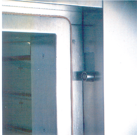
Detail view of the chamber. Note one of the three locking rollers which, by sliding upward, engage the three wedge-shaped lugs.
